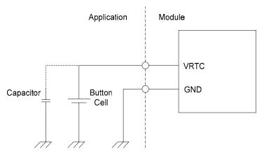
Figure 5.20-1 VRTC connection
